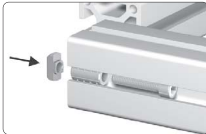
pre-mounting of the T-slot nut
