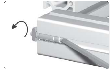
pre-mounting of the T-slot nut
