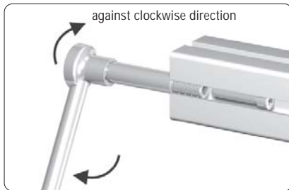
tighten the notching case (approx. 45° anti-clockwise turn)
