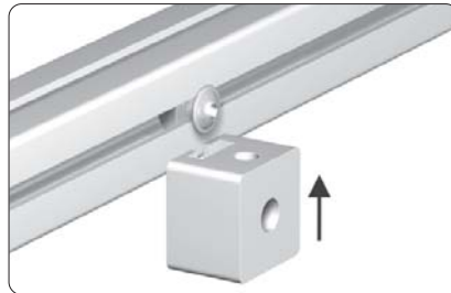
attach the connecting block
