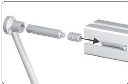
insert the cap head screw and the notching case into the slot
