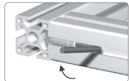
final tightening with socket spanner
