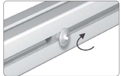
tighten the screw
