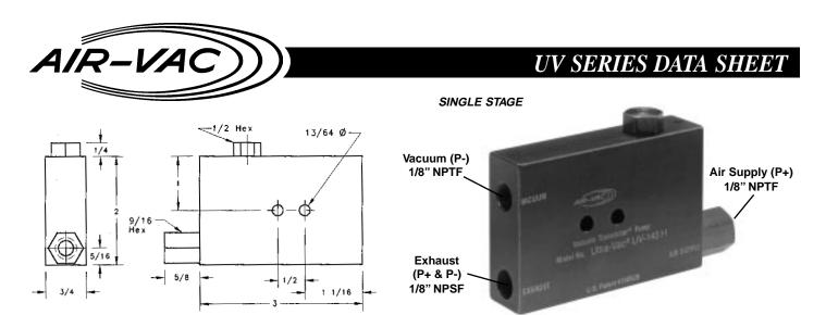
Ultra-Vac's design provides near perfect vacuum of 29.7"Hg. Used to evacuate chambers, degas liquids and in other processes requiring vacuum levels of 1/4"Hg absolute (8Torr). Ultra-Vac can be used as a first stage in applications requiring high vacuum to reduce operating time of expensive high vacuum pumping systems.
